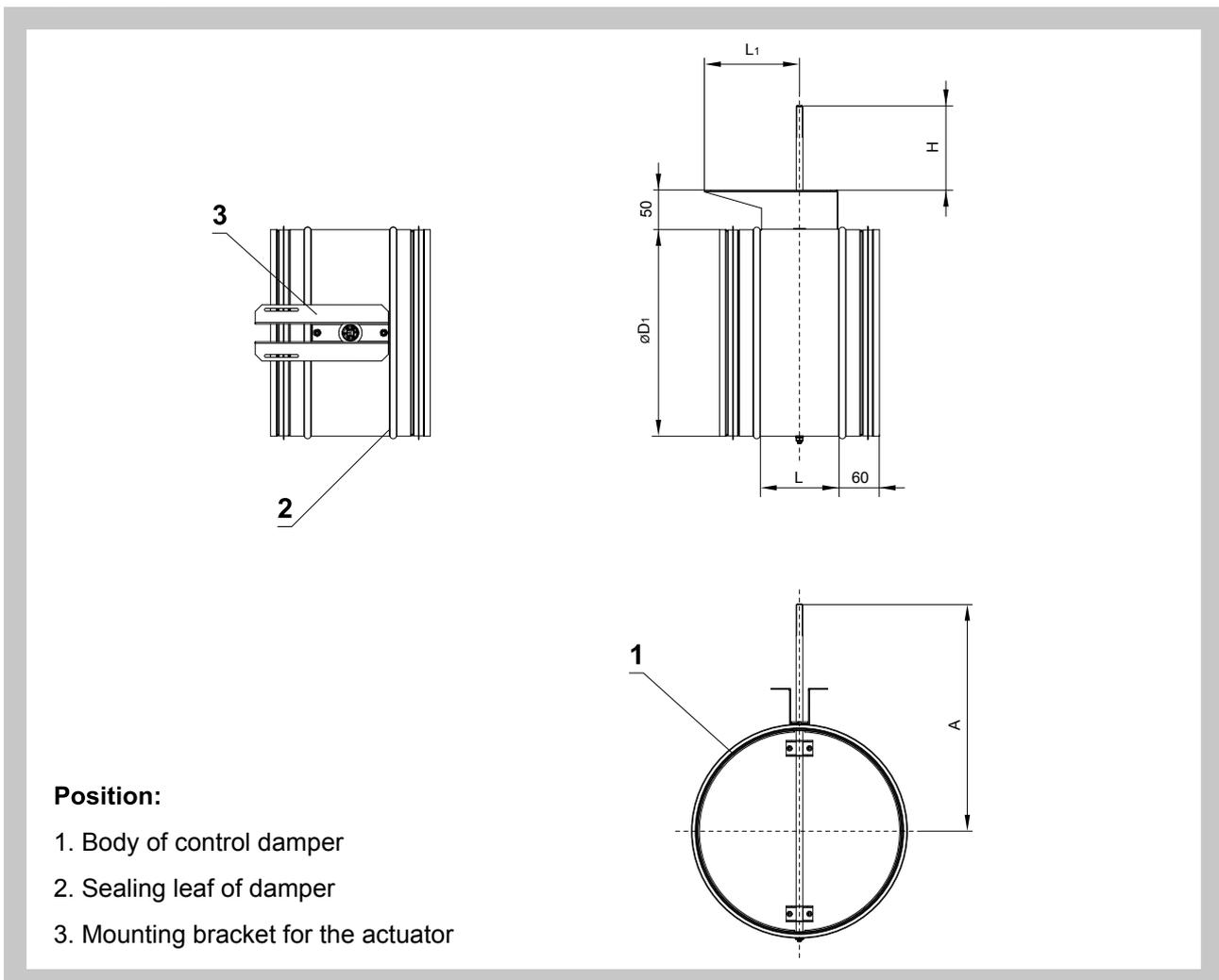
Dampers with actuator are set up by rectangular pin 10 mm.
