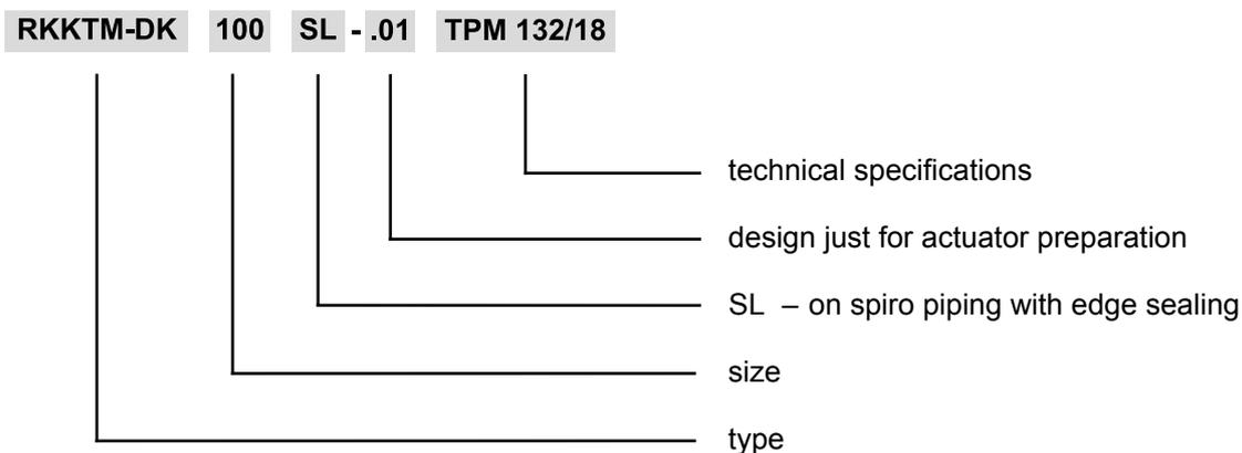
It is necessary to talk with the manufacturer regarding orders for versions with a different type of actuating mechanism.
